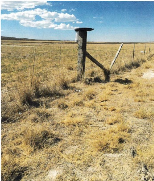
Figure 2. Typical mounting of a bulk deposition sampler. This sampler is located on Antelope Island of Great Salt Lake.
