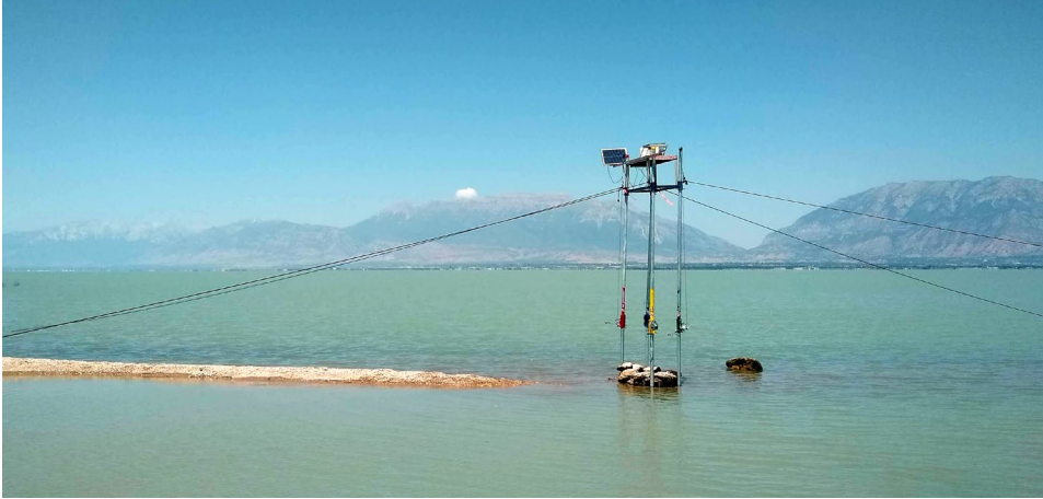
Figure 15. Photo of AD sampler installed at Bird Island in the south-central part of Utah Lake. The table was about 5 m above the water surface. The solar panel was mounted on a stainless-steel bar extending from the table surface to about 2.5 m from the sample buckets to prevent splash from reaching the sample buckets. The sampler was secured by guywires and weights extending approximately 50 m from each corner.
