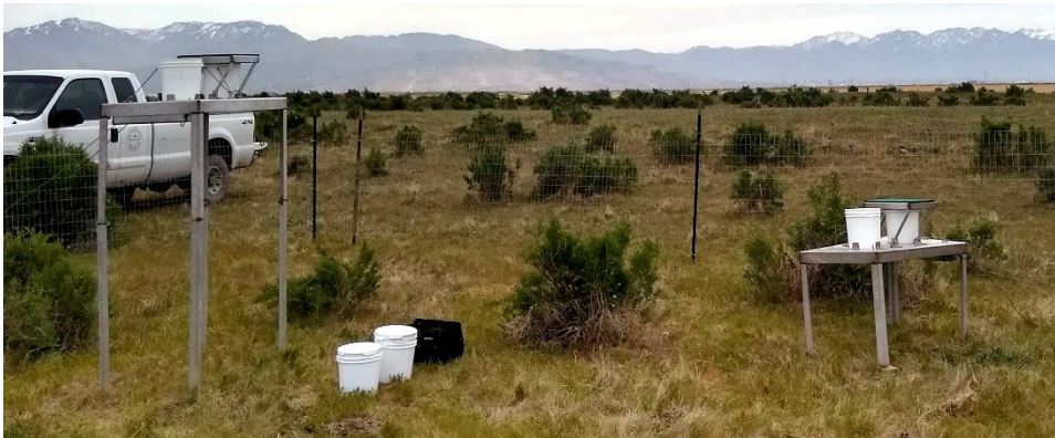
Figure 16. High (~2-meter) sample table on the left and the low (~1-meter) sample table on the right. The solar panels were mounted on T-posts located 5 m from the tables. Note green miner's moss attached to the surface of the lid covering the wet-side buckets.
