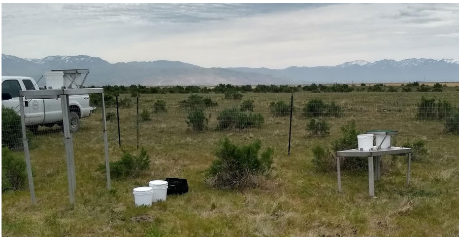
Figure 3. Photograph of AD samplers located within the Ambassador Duck Club. The samplers are equipped with a solar-powered battery that powers a moisture sensor and actuator/motor that shifts the lid to expose the “wet side” bucket and cover the “dry side” bucket when rain or snow occurs. When the moisture sensor dries (a few minutes after a rain event), the actuator returns the lid to cover and preserve the rain sample. The sampler on the right was the original design (top of bucket at about 1.2 m above the ground). After concern expressed by the Utah Lake Science Panel, the legs were extended in 2020 to situate the top of the bucket at 2 m above ground level (sampler on left).
